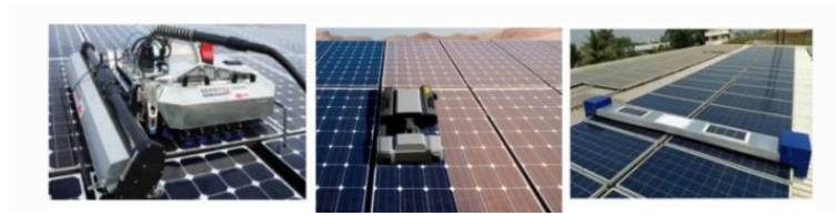
Figure 1: PV panel dry cleaning using robot (Bagnold 2012)
