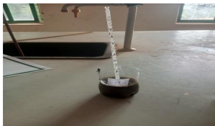
Plate 4: Determination of Bio-Digester A Temperature Digester B (Cow Dung and Neem Seed)
