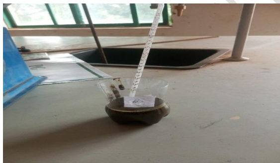
Plate 7: Determination of Bio-Digester B Temperature Digester C (Cow Dung and Groundnut Shell)
